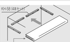
溝寸法:幅10.5mm×深さ17mm
